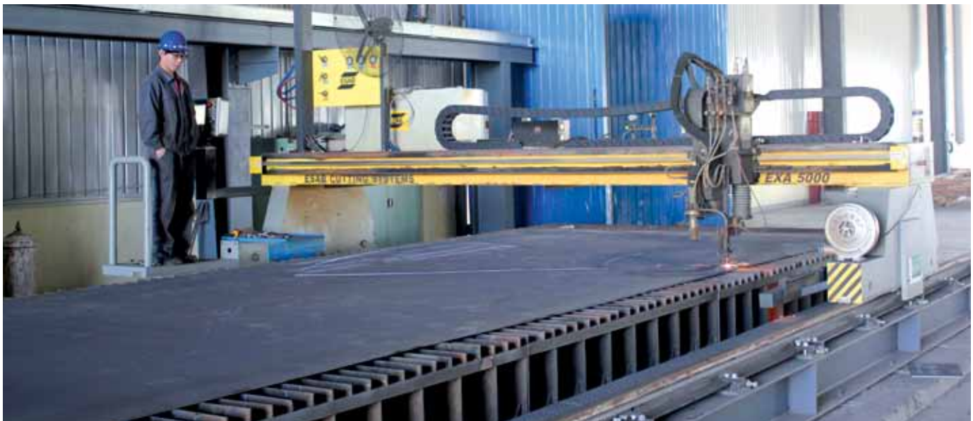
Checking of plates and precision cutting with CNC Oxy-Plasma machine. Thicknesses up to 110 mm
