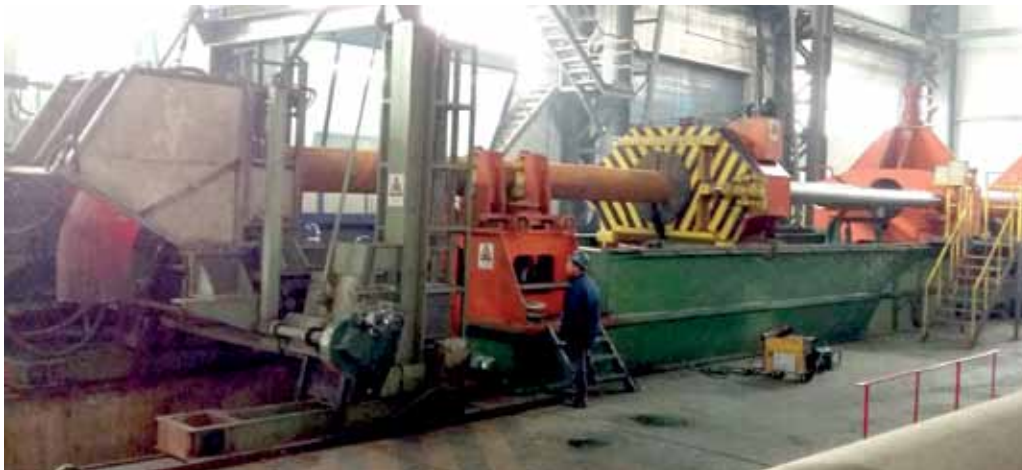
The larger mandrel bending: 900 tons pushing capacity, elbows up to 44" and bends (3D, 5D, 7D) up to 44"
