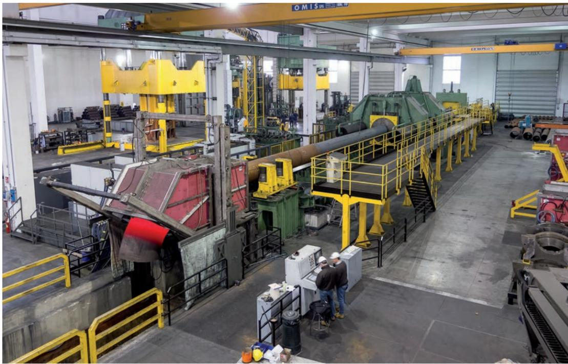
*A large-dimensions induction mandrel and bending machine capable of unequalled production and performances*
