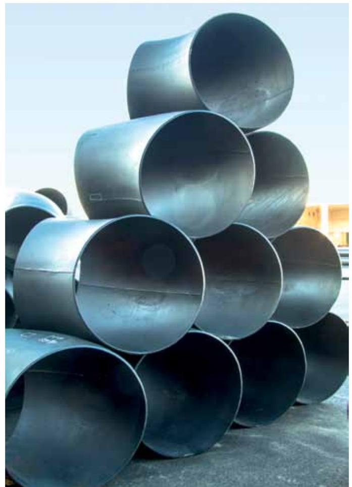
*Seamless pipes, heavy wall elbows and large diameter elbows for the power industry*
